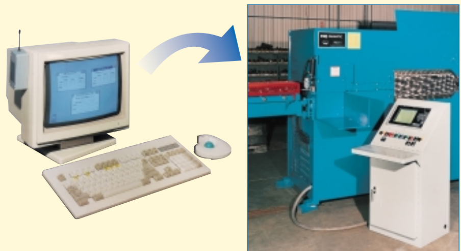
Figure 4: A bending machine controller obtains information directly from the office database
